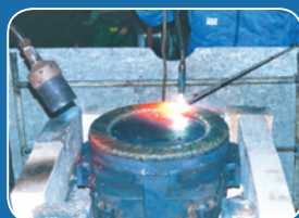
Stellite Overlay Welding
