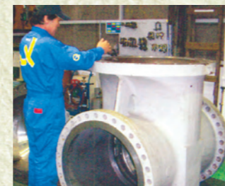
Overhaul of gate valves
