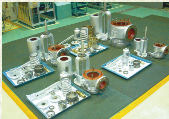
Overhaul of safety valves
