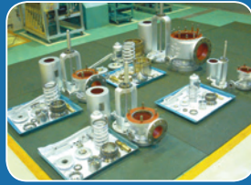
Maintenance of Safety Valves
