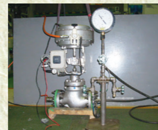
Leakage testing of control valve seat
